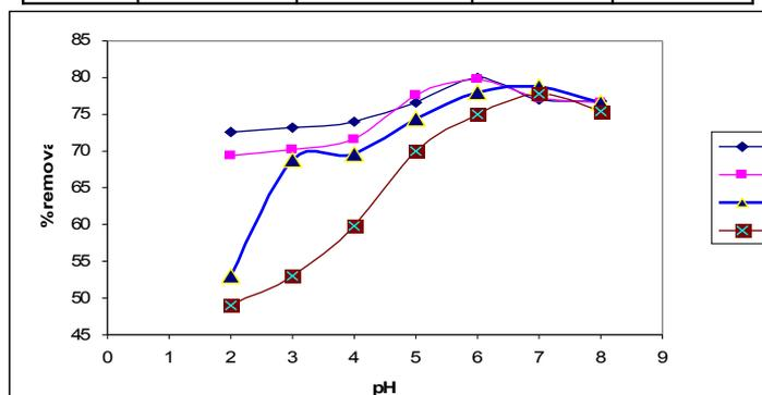
**Figure. 2 %Removal curve for Cu, Zn, Cd and Pb**
