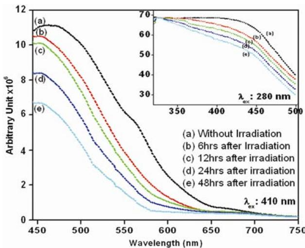
Fig. 2—Spectrum at 410 nm excitation shows a decrease in the fluorescence intensity with increase in time of exposure using mercury arc lamp [Inset shows the spectrum at 280 nm excitation]
