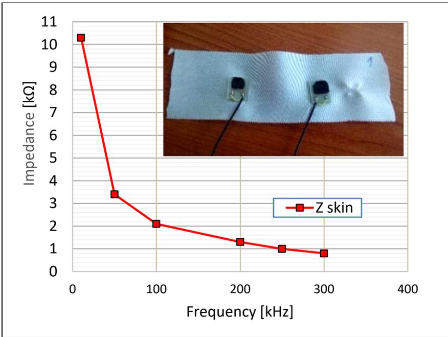
Figure 6. Skin interface bio-impedance response with frequency, for dry polarizable bio-impedance sensors S1 (PCB substrate with polypyrrole/Ag NP).
