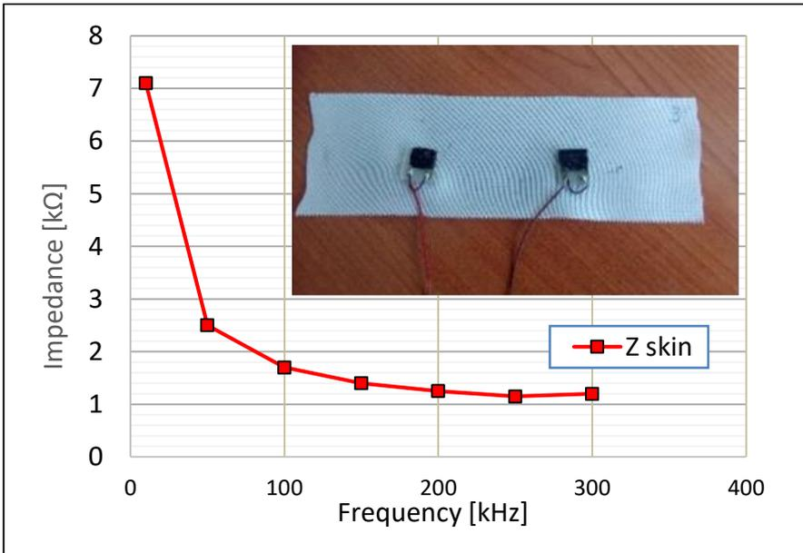
Figure 7. Skin interface bio-impedance response with frequency, for dry polarizable bio-impedance sensors S2 (PCB substrate with polypyrrole).
