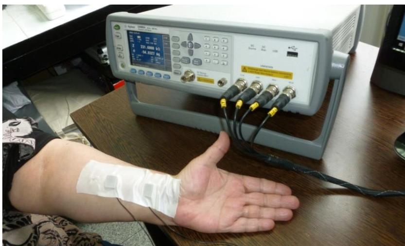
Figure 9. Test bench for measurements of the bio-impedance.
