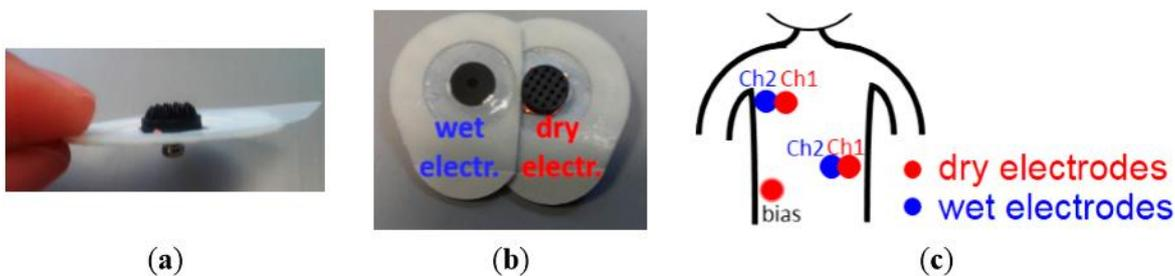
**Figure 3. (a) Conductive polymer dry electrode connects with gel removed wet electrode; (b) a pair of wet and dry electrode; (c) electrode locations for ECG measurements [27].**
