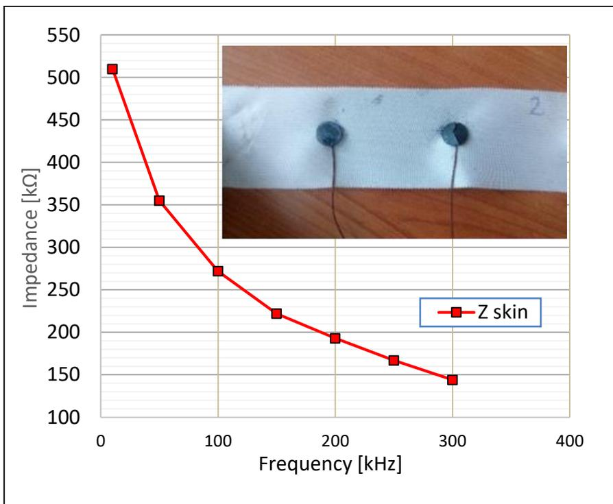
Figure 8. Skin interface bio-impedance response with frequency, for dry polarizable bio-impedance sensors S3 (disc with polypyrrole).
