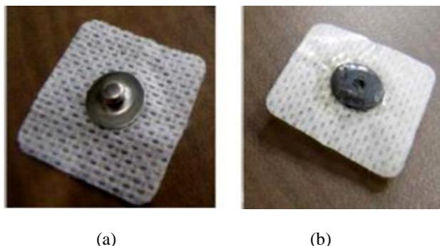
**Figure 1. (a) Ag/AgCl electrode (electrode's snap side), (b)Ag/AgCl electrode (electrode's skin side) [25].**
