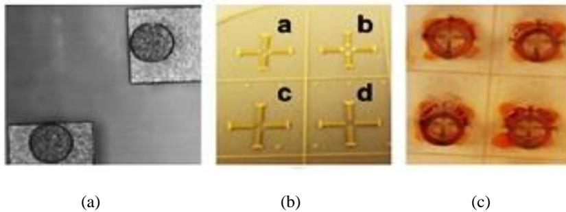
**Figure 4. Optic image of a microelectrode device with 2 lithographically defined electrode sensors; (a,b) photograph of four gold plated microelectrode devices on a glass wafer; (c) photograph of electrodes with cloning cylinders attached using photoresist as adhesive [22].**
