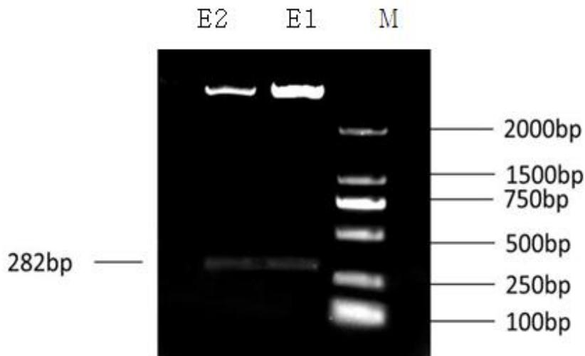
Fig. 5. Double digestion of recombinant vector pET30a-CsSUBP with restriction enzymes. E1, E2: Double digestion products; M: DNA marker DL2000
