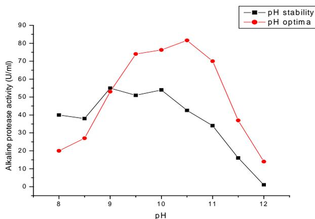
**Figure 3.pH optima and pH stability for purified alkaline protease**
