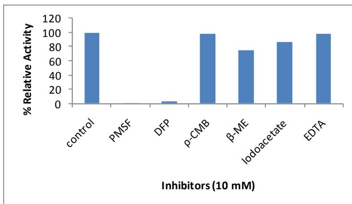
Figure 4. Effect of inhibitors on purified alkaline protease activity
